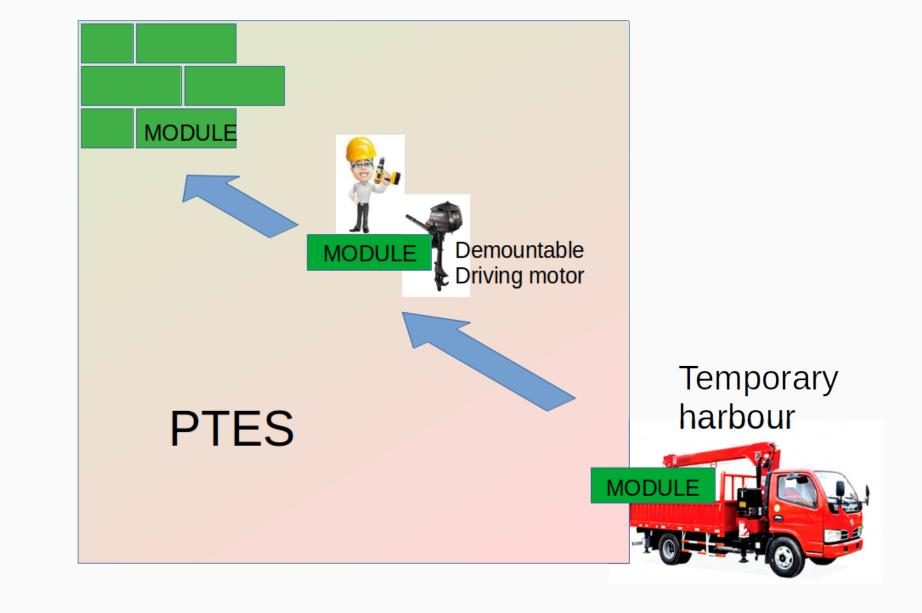
The modules are pre-fabricated in a factory and can be efficiently transported in 7.2x2.4m format. The trucks are unloaded at the "temporary harbour". The modules are equipped with a driving motor and put on the water with a small 2 ton crane. A worker can navigate the module exactly against the already built pontoon, before fixing with an extra strip polyurea.
