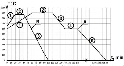
Fig. 4. The optimum temperature-time modes of block (A) and granulated (B) foamed slag glass' synthesis. 1 - calefaction, 2 – foaming, 3 – quenching (rapid cooling) with structure stabilization, 4 – additional thermal stabilization, 5 – annealing (gradual cooling).
