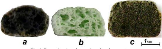
Fig. 1. Foam glass based on various foaming agents: a – anthracite, b – chalk, c – glycerol mixture
