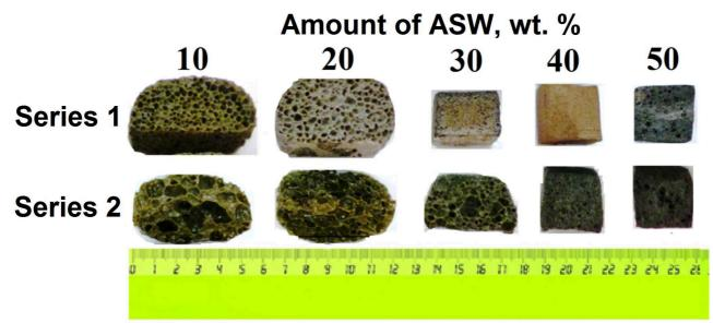
Fig. 2. Foamed slag glass with different contents of ASW
