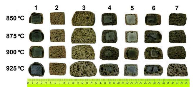
Fig. 3. Influence of the type and amount of foaming agents on the structure of foamed slag glass
