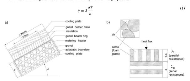
Figure 1 a) schematic representation of the experimental setup for measurement of the thermal conductivity of gravel beds. b) gravel phases (top) and Krischer model (bottom)
