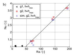
Figure 5: Influence of natural convection with upward heat transfer on gravel 1 (compressed, h = 0.235 m) and gravel 2 (uncompressed, h = 0.3 m). Comparison between simulation (sim.) and experimental results. a)  $\lambda$ -Nu vs  $\Delta$ T. b) Nu vs Ra for  $\gamma = 180^{\circ}$
