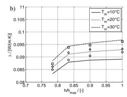
Figure 3: Measured data of thermal conductivity of gravel 1 and results calculated with the Krischer-model for different mean temperatures and compression degrees (uncompressed gravel corresponds to h= 30cm)
