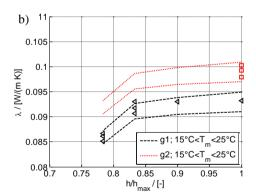
Figure 4: Comparison between thermal conductivity of gravels 1 and 2. a) thermal conductivity as function of the mean temperature. b) thermal conductivity range as function of compression degree with  $h_{max}$ =30 cm. The gravel 2 range (dotted lines) is traced assuming the both gravels presenting similar behaviours.
