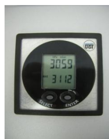
Display segments of the digital manometer Leo 1 and the manometer at the air pycnometer
