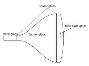
1: Main glass components of a typical cathode ray tube
