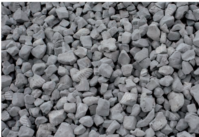
Figure 2. Foamit- foamed glass aggregate's typical granular shape
