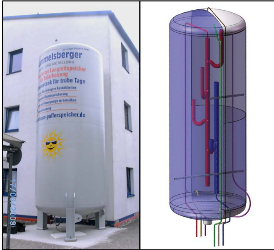
Figure 7.1: Layout of the real-size storage tank prototype: Photograph of the tank (a), sketch of the inner container with supply pipelines and stratification device (b).
