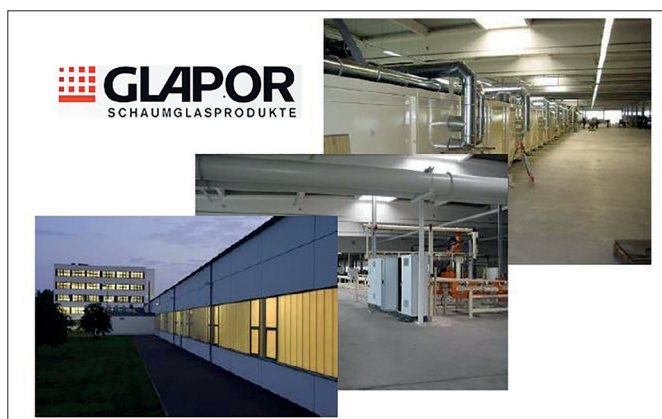
◀ Fig 1. Continuous foaming furnace and lehr for cellular glass.
