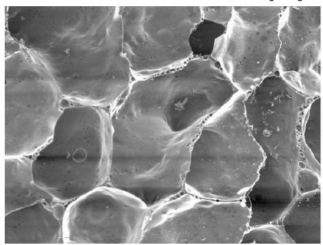
Structure of foam glass granules as seen through an electronic microscope
