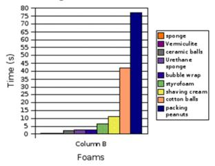
Figure 1. Average time required to change the temperature of a foam by one degree Celsius for each tested foam
