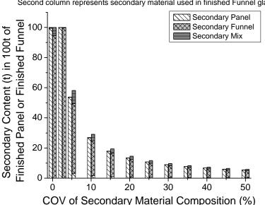
Figure 7. Secondary glass content in finished panel or funnel for identical baseline secondary and new glass compositions and +/- 10% new glass compositional specifications.
