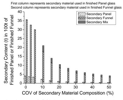
Figure 6. Secondary glass content in finished panel or funnel for typical secondary and new glass compositions and +/- 25% new glass compositional specifications.
