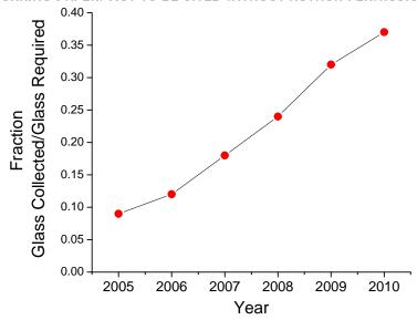
Figure 4. Ratio of secondary glass collected to new glass required.
