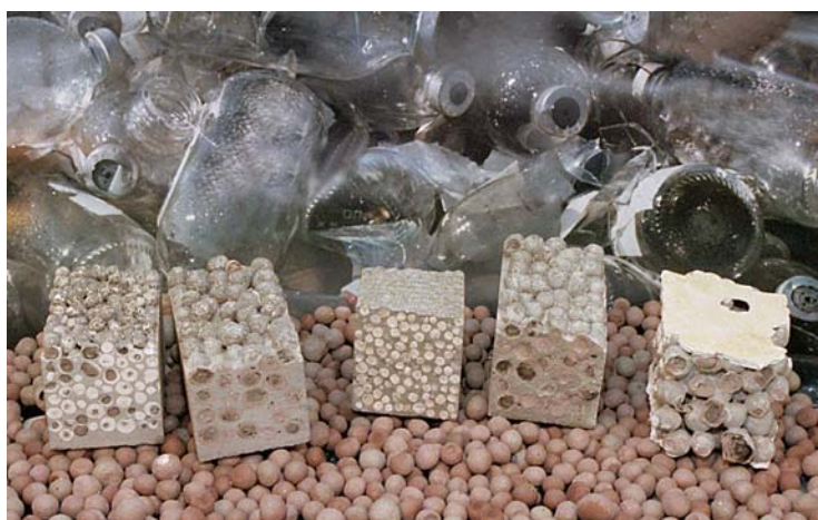
From glass, to pellets to products (Geofil-bubbles)
