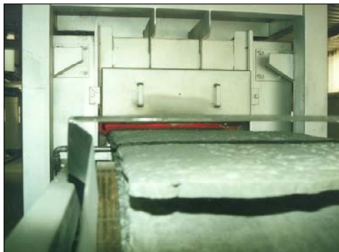
Figures 7 and 8 - Foam glass exiting the furnace and being used for a loose aggregate floor insulation
